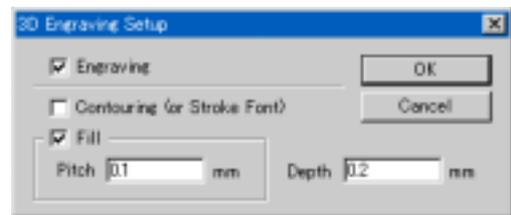
6. Click [OK]. The view changes to the 3D screen and shows the tool path for engraving in red.
