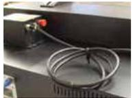
11. Plug the anti-static bar into the power supply box. Secure yellow grounding wire between hex nuts.
