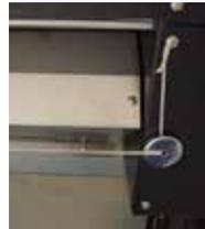
4. Slightly unscrew the screw that appears on the back of the printer and tie the cord around it once and then tighten the screw.
