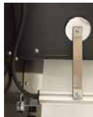
8. Affix one fastener to each end of the bottom of the power supply box. Attach the mating component to each of the two fasteners.
