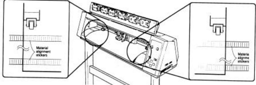
**#3 Loading cartridges:** Remove cartridges from box. There is a small cardboard piece to keep the cartridges taut. Remove this piece and load into any cartridge holder slot with the B side out. The Roland logo should not be visible when properly loaded. It may be necessary to re-tension cartridge ribbon after installation into the holder.
