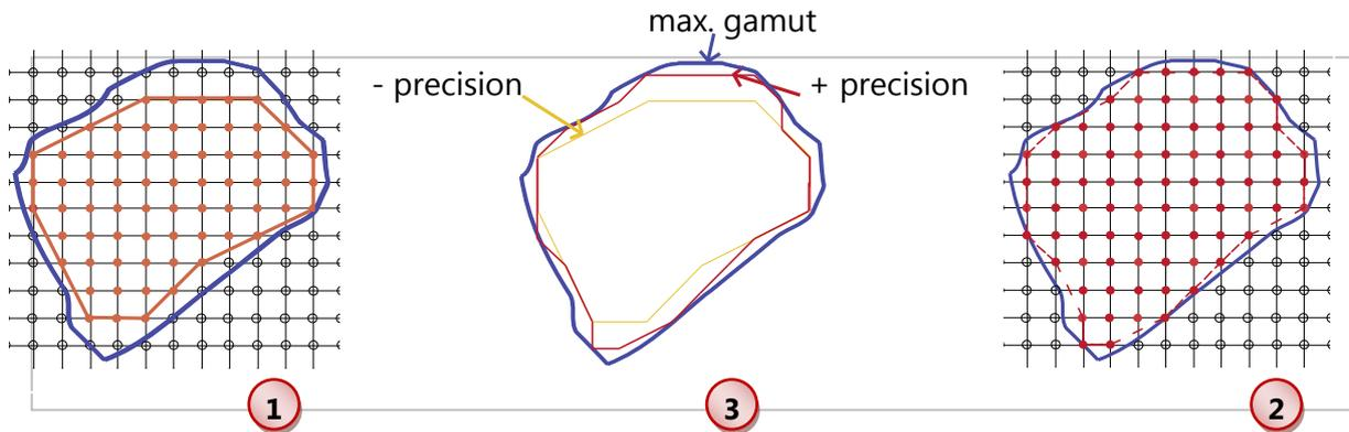
To further describe how the number of printed patches affects the profile, the images 1 + 2 show heavily simplified graphics of the maximum LAB gamut (outer blue line) and the device specific CMYK gamut (inner line). In image 1, less grid points are selected than in image 2. Hence the gamut in image 2 is described more accurately than the one in image 1 and can therefore be used more efficiently (see image 3).
